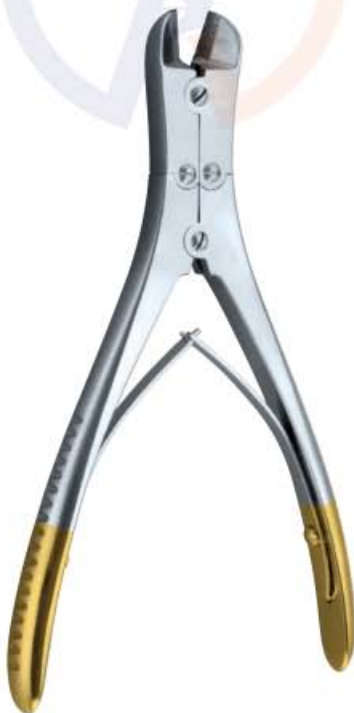
Side Wire Cutter 09-1463-18 18cm for hard wires up to 1.5mm, for soft wires up to 2mm 09-1464-22 22cm for hard wires up to 2.2mm, for soft wires up to 2.8mm tungsten carbide inserts
