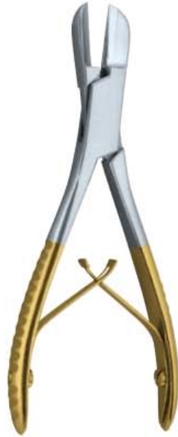
Wire Cutter 09-1460-15 15cm for hard wires up to 1mm, for soft wires up to 1.5mm tungsten carbide inserts
